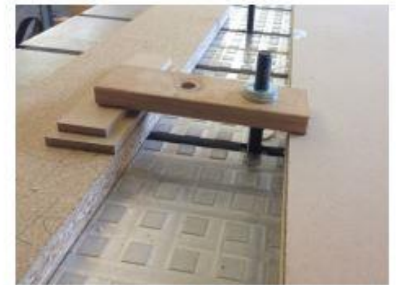
Use washers to protect bolt thread (if necessary)
