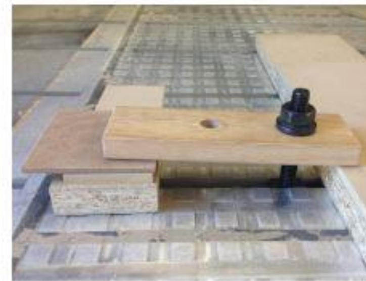
Position the clamp fingers with step blocks
