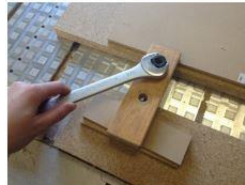
Tighten the bolts to secure the stock
