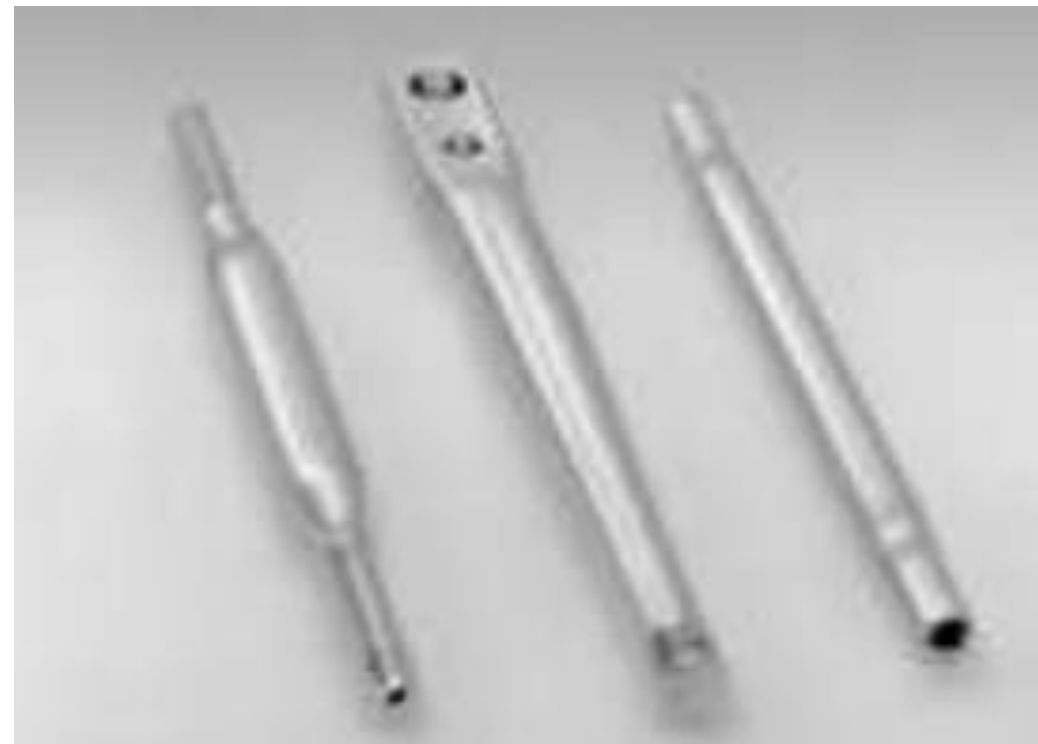
Swaging at the ends, ready for next forming process.
